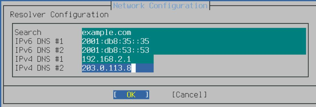
Figure 59. Configuration du DNS
